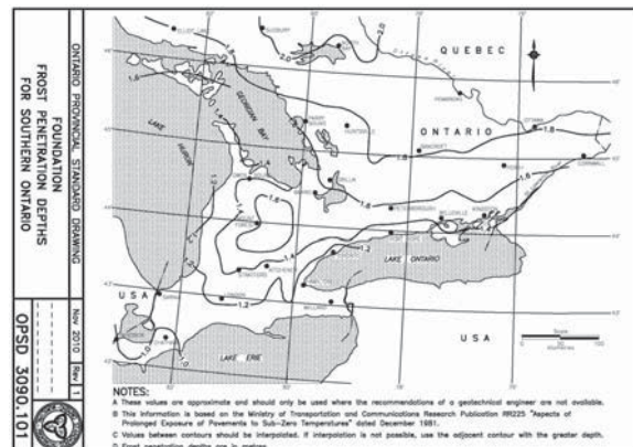
Figure 1. Design Contours of Frost penetration (Southern Ontario)
